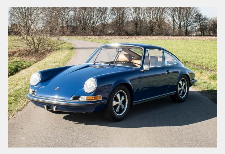
From the **24 Hours of Le Mans** to **grass-roots Motorsport**, the **911** was simply the car to have. For 1970, the **'C-Series' 911** was introduced with a larger bore to give a capacity of 2165cc, producing 125bhp and now badged as a «T». Alterations to the suspension geometry improved the handling and added a bit more weight to the steering feel.
